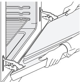
HINGE SLOT - Door removed
