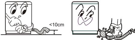
3. If the drain hose is too long, cut it at mid point. To make smooth drainage, cut the front end of the hose slantingly.
