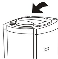
As the top lid opened, the Washer will automatically give an alarm and stop running, exclusively during supplying water and rinsing.
