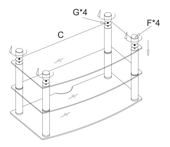
5. Put the rubber pads (G) on glass (C), then screw the feet (F) on the glass (C).
