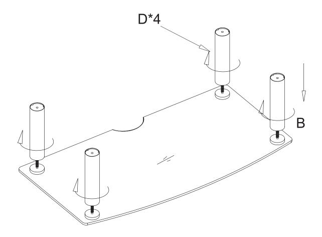
1. Turn glass (B) up side down, and screw 4 pillars to glass.
