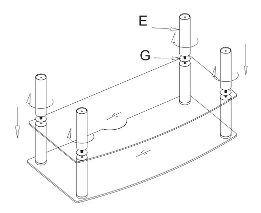
3. Put the rubber pads (G) on glass (C), then screw pillars (E) on the glass (C).
