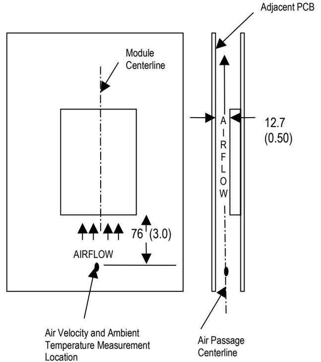
**Wind Tunnel Test Setup**
