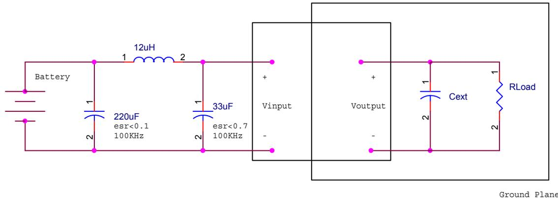
The input reflected ripple is measured with a current probe and oscilloscope. The ripple current is the current through the 12uH inductor.
