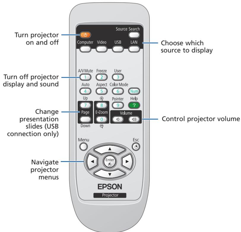
You can use the remote control to operate the projector. With the USB cable, you can use the remote as a wireless mouse. For more information on using the remote control, see your *User's Guide*.
