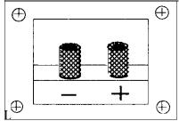
Remember: switch the amplifier to STANDBY before attempting any connection. Do not turn the amplifier ON until all connections are completed!
