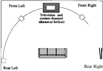
In a home theater environment, placement for the speakers is closely tied to the location of your television. The diagram at left will provide you with the general layout of your home theater system, indicating the variety of positions for all the speakers. When setting up your system, try to avoid placing other furnishings between the speakers and your viewing/listening position or directly alongside the speakers as these can diminish sound quality
