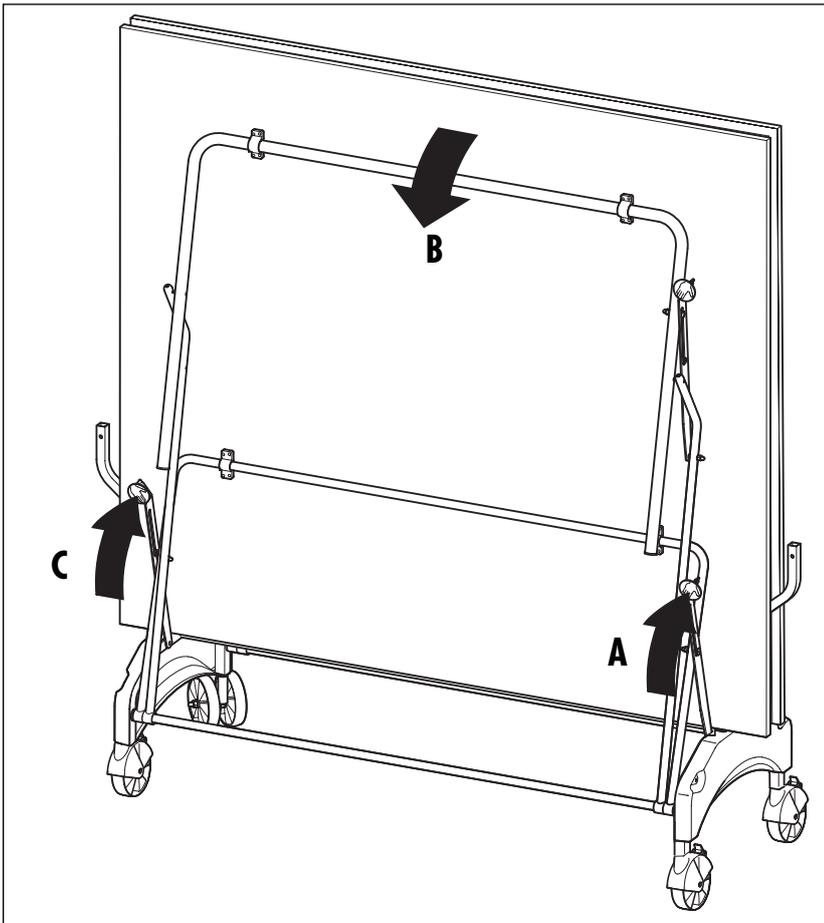
**USA** Press the right-hand tip lock. Hold the table firmly with one hand, press the left-hand lock and lower the table-half slowly into position. Never allow it to drop down!
