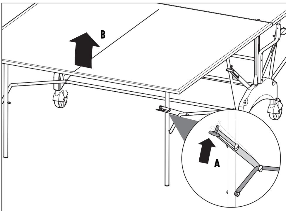
**USA** Press the locking lever up and lift the table half upwards. Continue to press the lever during the first part of the upward motion.
