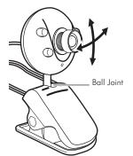
Rotate the ball joint to adjust the angle of view.
