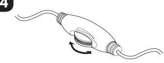
Use the switch on the cord to adjust the LED brightness on the webcam's face.
