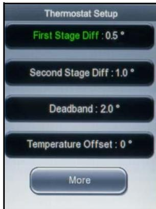
FIG. 49 Thermostat Setup screen (1 of 2)
