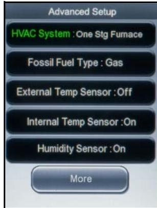
**FIG. 43** Advanced Setup screen (1 of 3)
