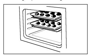
Do not place dishes or baking trays directly on the oven floor as it interferes with the oven air circulation and can lead to base burning; use the lower shelf position. However non critical dishes can be placed on the oven base when more space is required.
