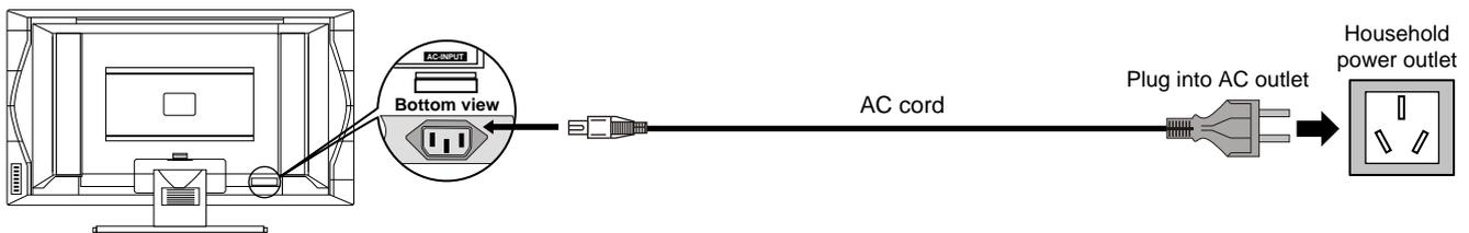
1. Connecting the female plug to the AC socket on the unit.
