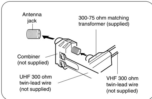
Connect the UHF 300 ohm twin-lead wire to the combiner (not supplied). Connect the VHF 300 ohm twin-lead wire to the 300-75 ohm matching transformer. Attach the transformer to the combiner, then attach the combiner to the antenna jack on the back of the TV/DVD.
