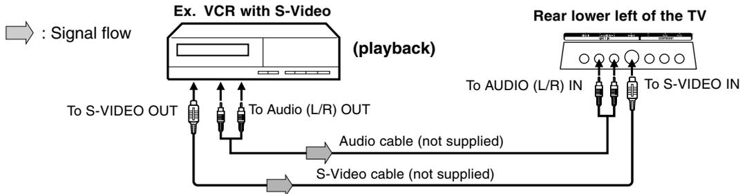
**Note:** When the S-VIDEO cable and the standard video cable are connected at the same time, the S-video cable takes precedence.
