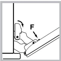
2. Use a screwdriver to lift up and turn the small levers **F** located on the two hinges (see diagram).
