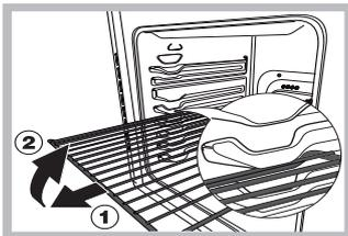
**WARNING!** The oven is provided with a stop system to extract the racks and prevent them from coming out of the oven (1). As shown in the drawing, to extract them completely, simply lift the racks, holding them on the front part, and pull (2).
