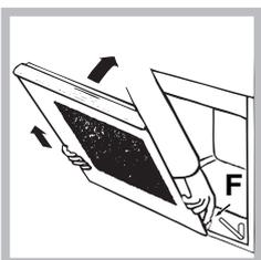
3. Grip the door on the two external sides and close it approximately half way. Unlock the door by pressing on the clamps **F**, then pull the door towards you lifting it out of its seat (see diagram).
