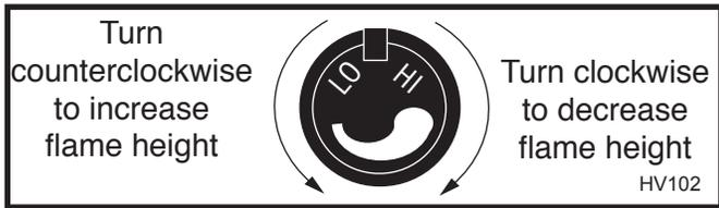
Fig. 13 Flame adjustment knob for Honeywell valve.
