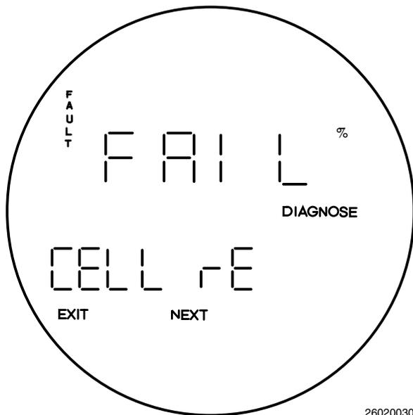
Figure 6-11. Fault 7, Reversed O<sub>2</sub> Cell
