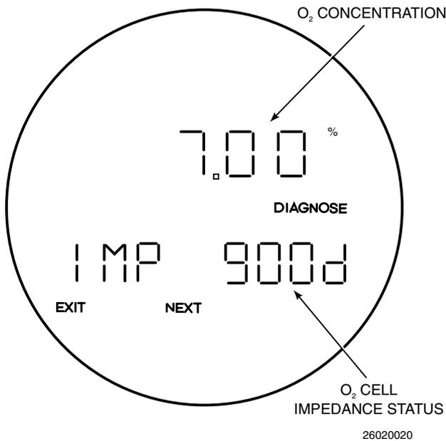
Figure 3-23. CELL IMPEDANCE
