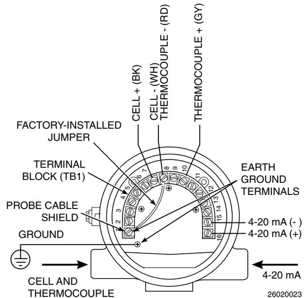
**Figure 6-4. Model 3081 Transmitter Terminal Block**
