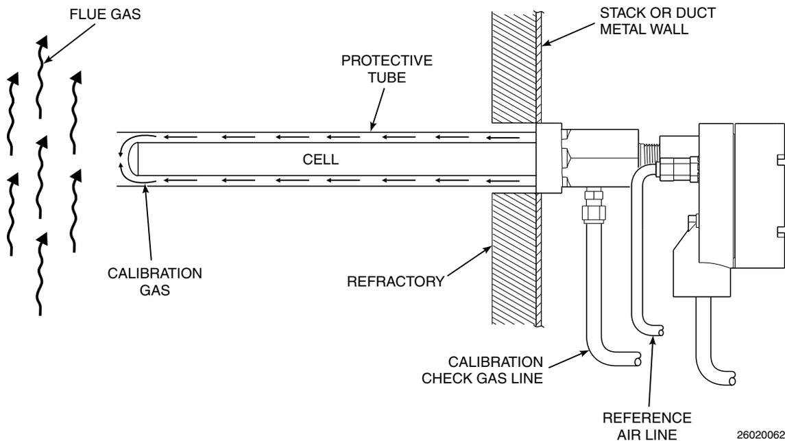
**Figure 3-3. Proper Calibration Check Gas Flow Rate**
