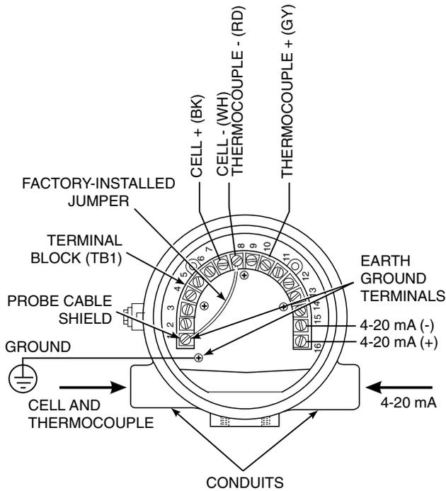
NOTE: RUN CELL AND THERMOCOUPLE SIGNALS IN SEPARATE CONDUIT FROM 4-20 mA LINE.
