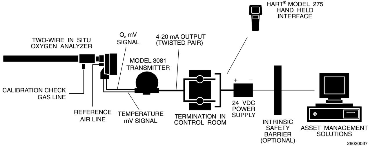
Figure 1-2. Two-Wire In Situ Oxygen Analyzer HART Connections and AMS Application
