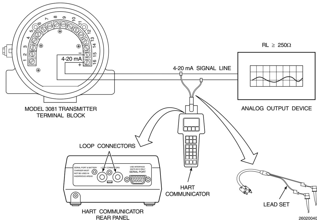
**Figure 4-1. Signal Line Connections,  $\geq 250$  Ohms Lead Resistance**
