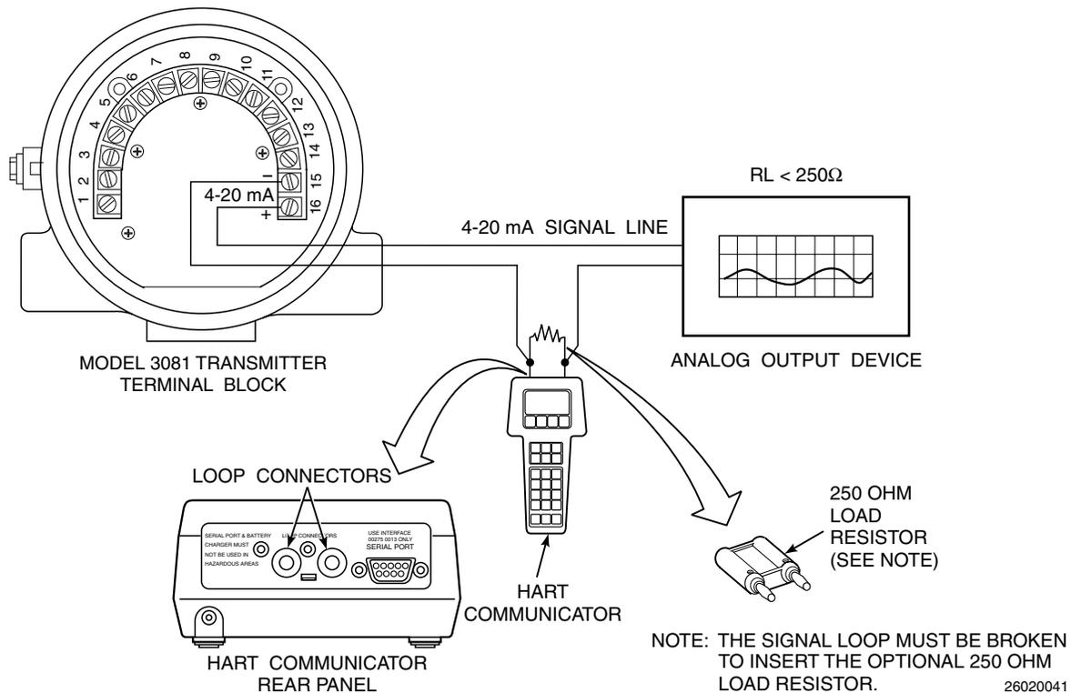
**Figure 4-2. Signal Line Connections, < 250 Ohms Lead Resistance**
