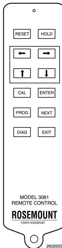
**Figure 3-6. Infrared Remote Control (IRC)**
