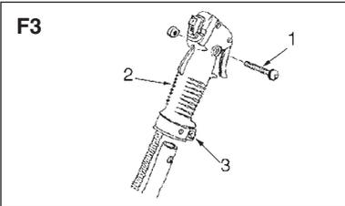
3. Remove the screw (F3-1) from the right grip (F3-2) and put the grip onto the right handle. Align the positioning holes and put the screw through them. Fasten the clamp. (F3-3)
