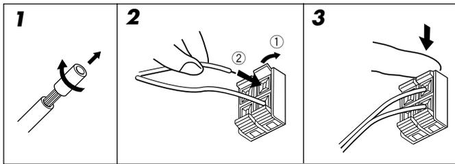
For each speaker, connect the (+) and (-) terminals on the rear panel to the (+) and (-) terminals marked on the speakers.
