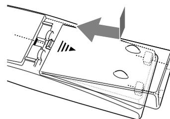
If the range or effectiveness of the remote control decreases, replace the batteries. Use two R6P(SUM-3)/AA(15F) type dry-cell batteries.
