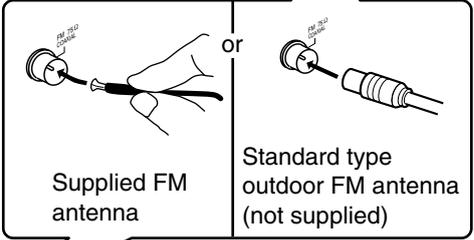
Supplied FM antenna or Standard type outdoor FM antenna (not supplied)
