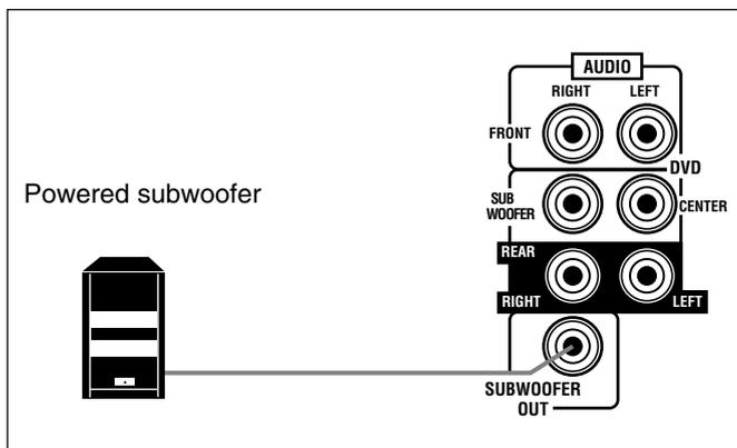
Connect the input jack of a powered subwoofer to the SUBWOOFER OUT jack on the rear panel, using a cable with RCA pin plugs (not supplied).
