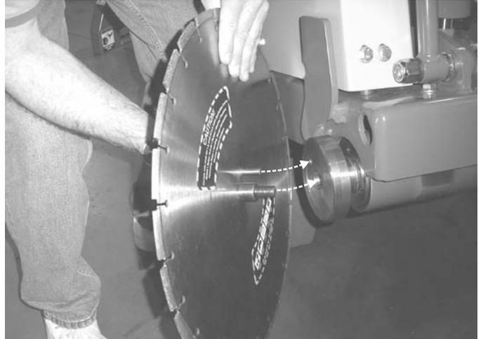
**Figure 11. Aligning Flange Pin Through Blade**
