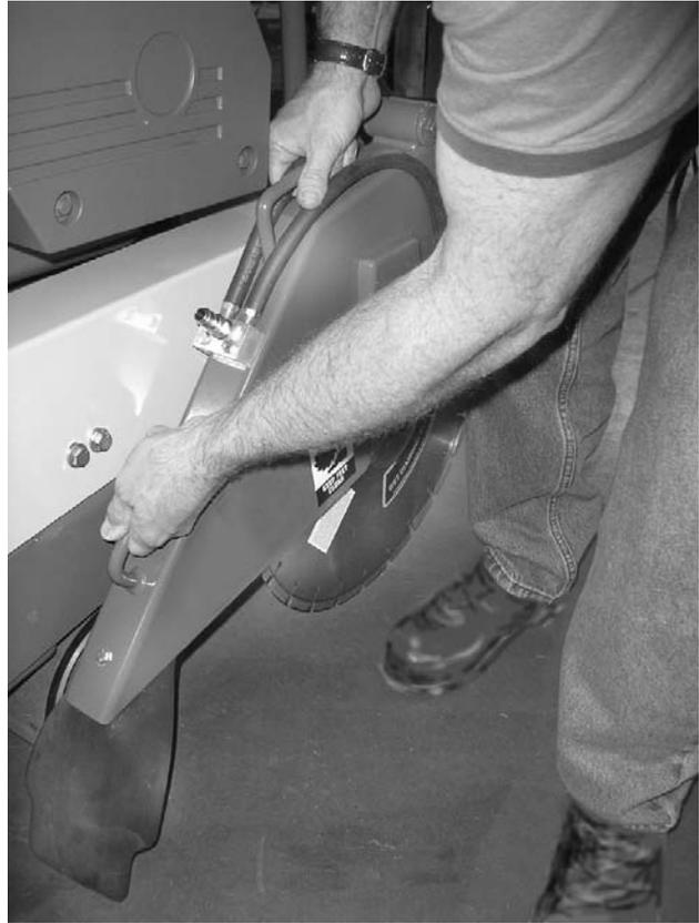
Figure 16. Removing The Blade Guard
