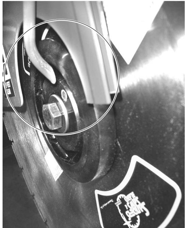
Figure 21. Large Blade Guard Water Tube
