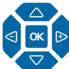
**Navigator:** this comprises four direction keys and one central key.
