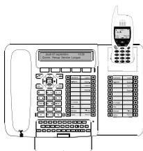
The extension module lets you enhance your set by adding a further 20 programmable keys. You can add up to two extensions, giving you a total of 60 programmable keys.
