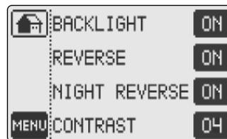
❑ **BACKLIGHT:** Select between automatic and permanent backlight for the screen.
