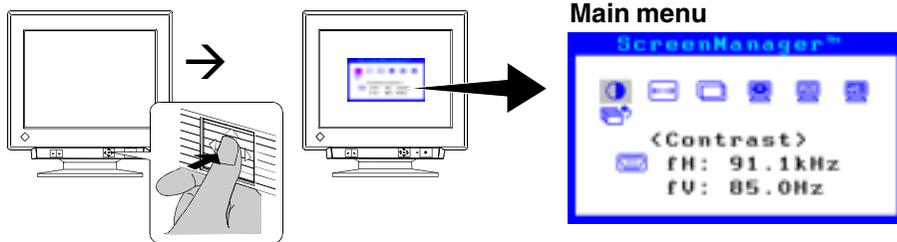
Main menu displays the current connector type and frequency of the input signal.
