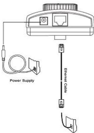
Please verify that your product package contains all the accessories listed in the foregoing Package Contents. Depending on the user's application, an Ethernet cable may be needed. The Ethernet cable should meet the specs of UTP Category 5 and not exceed 100 meters in length.
