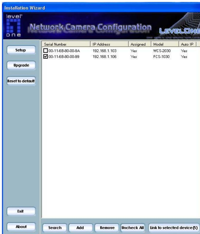
Installation wizard allows you to setup or upgrade multiple devices (of the same model) at the same time. If you selected different models, then the buttons will be disabled. There are five buttons on the bottom of the main page, and five buttons on the left panel of the main page.
