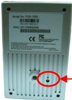
button in the back of the Network Camera. It is used to reset the system or restore the factory default settings. Sometimes resetting the system sets the system back to normal state. If the system problems remain after reset, restore the factory settings and install again.
