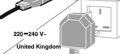
The plug is fitted with a fuse which protects your television. If your television does not work, the fuse may be blown. In this case, replace it with an identical 5 Amp ASTA or Ir BSI (BS 1362) certified fuse.
