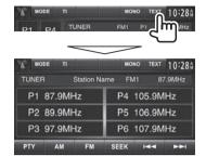
The preset list containing the station names for FM RBDS (when PS signal is coming in) is displayed.
