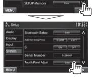
Touch the center of the marks at the lower left and at the upper right as instructed.
