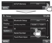
The security indicator on the monitor panel flashes when the vehicle ignition is off.
