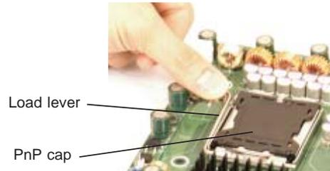
2. Gently lift the load lever to open the load plate.
