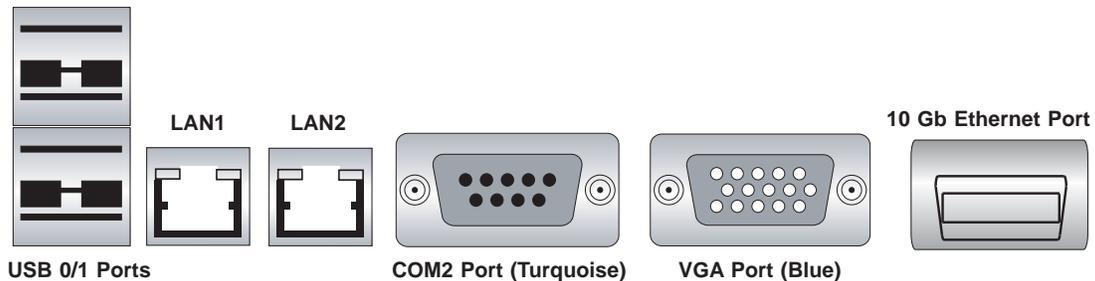
**Note:** The 10 Gb Ethernet port is included on the X7DCT-10G (6015TC-10G) only.
