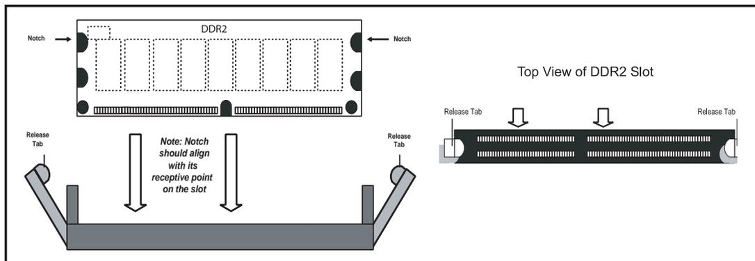
To Install: Insert module vertically and press down until it snaps into place. Pay attention to the bottom notches.
