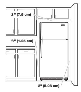
To ensure proper ventilation for your refrigerator, allow for a %" (12.7 mm) space on each side. Allow 3" (7.5 cm) of space between overhead cabinets and refrigerator top. Allow at least 1" (25.40 mm) between back of cabinet and the wall. If your refrigerator has an ice maker, make sure you leave some extra space at the back for the water line connections.
