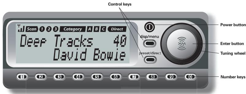
The XMCommander unit has a power button, two control buttons, tuning wheel, enter button and 10 number keys.
