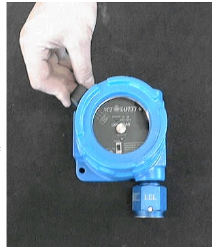
Figure 15 - Magnetic Reed Switch Activation
