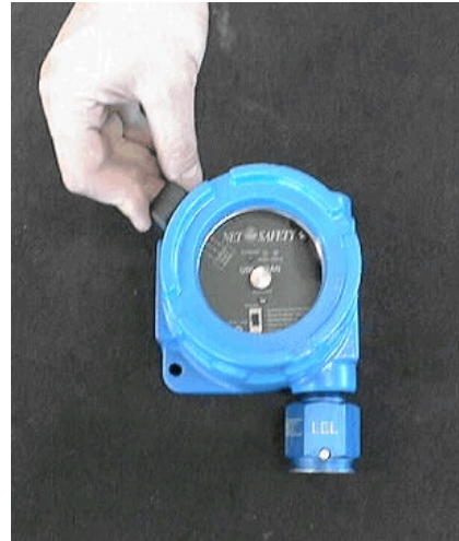
Figure 17 - Magnetic Reed Switch Activation
