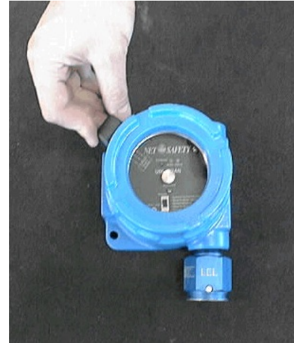
Figure 14 - Magnetic Reed Switch Activation
