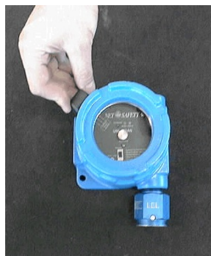
Figure 16 - Magnetic Reed Switch Activation
