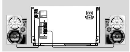
Connect the speaker wires to the SPEAKERS (FRONT) terminals, right speaker to "R" and left speaker to "L", coloured (marked) wire to "+" and black (unmarked) wire to "-". Fully insert the stripped portion of the speaker wire into the terminal as shown.
