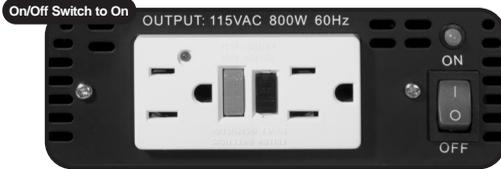
2. Plug a test lamp into the outlet.
