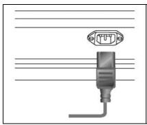
Plug the power cable supplied into the power connector of the LCD TV.
