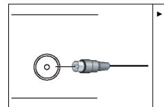
Connect an antenna cable to the antenna connection of the plasma TV and to the TV antenna socket.
