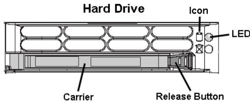
Press the red release button to release the handle on the carrier, and then extend the handle fully and pull the carrier out towards you. Replace the failed drive with your spare replacement drive.
