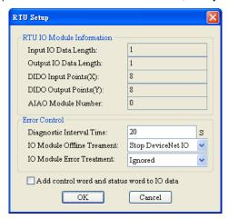
(12) Set up the parameters in RTU-DNET and confirm its I/O information.
