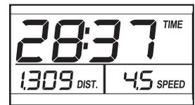
To reset the displays, press the Stop button, remove the key, and then reinsert the key.
