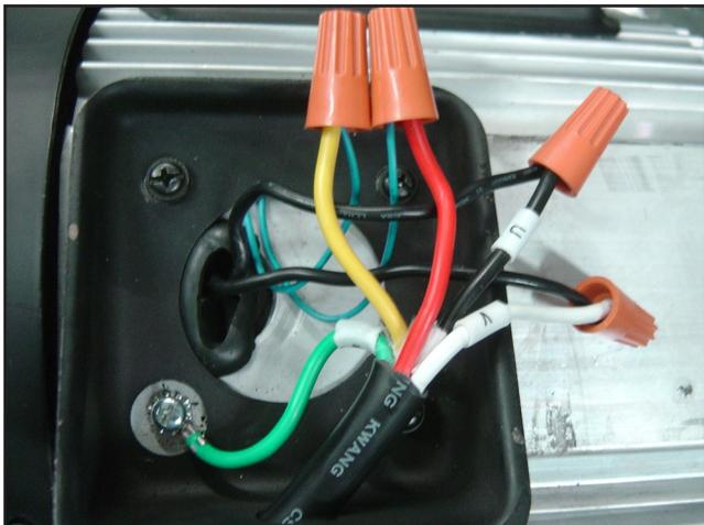
Figure 18. Motor wiring.
