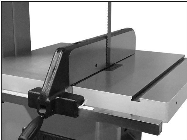
Figure 11. Fence flush with blade.
