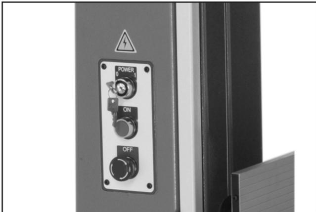
**Figure 8.** G0513X2 switch disabling key and ON/OFF switch.
