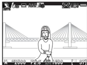
**4** Recompose the picture while keeping the shutter release button pressed halfway.
