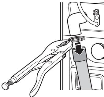
2. Slide drain hose onto washer connection.
