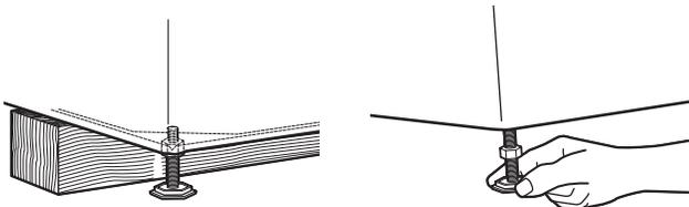
If the washer is against a wall, move the washer out slightly before tipping back. If the washer is not level, first prop the front with a wooden block and adjust the front feet height moving the hexagonal plastic part as necessary. Repeat to adjust back feet.
