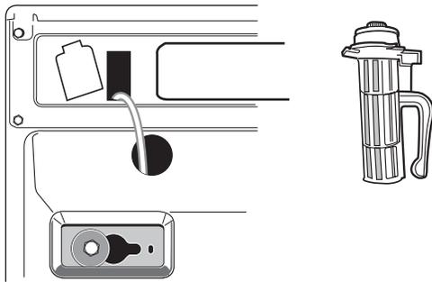
1. On the back of the washer, loosen the 4 transport bolts using a 13 mm wrench.
