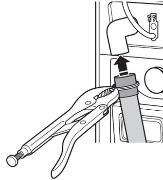
3. Once drain hose is in place, release pliers.
