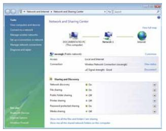
3 Click Connect to a network on the left of the window. The Connect to a network dialog box opens.
