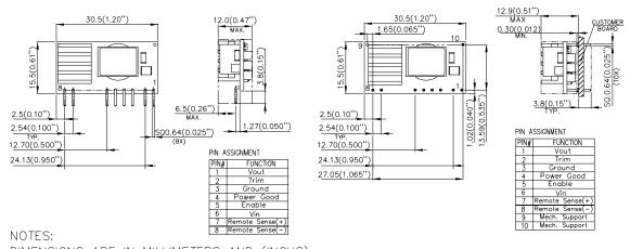
DIMENSIONS ARE IN MILLIMETERS AND (INCHS) TOLERANCE: X.X mm±0.5 mm(X.XX in.±0.02 in.) X.XX mm±0.25 mm(X.XXX in.±0.010 in.)
