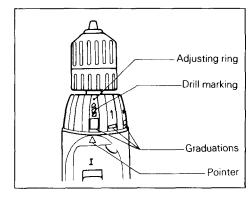
material to determine which torque level is required for a particular application.
