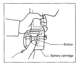
•Do not use force when inserting the battery cartridge. If the cartridge does not slide in easily, it is not being inserted correctly.
