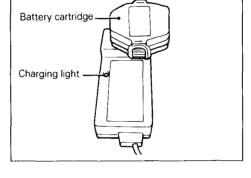
Insert the cartridge fully into the port so that it rests on the charger port floor.
