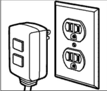
**Step 1** Plug the Ground Fault Circuit Interrupter (GFCI) into a working outlet.
