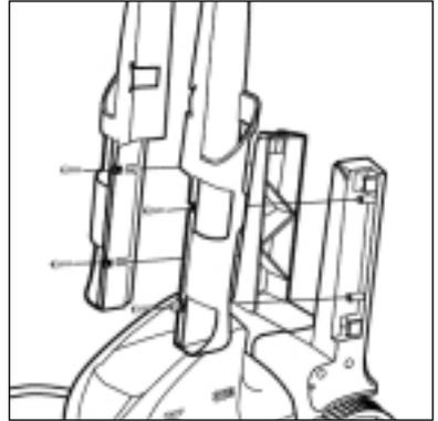
**Step 2** Slide the handle onto the mobile adapter brackets as shown, insert screws and tighten.
