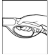
**Step 4** Press trigger to release water pressure.
