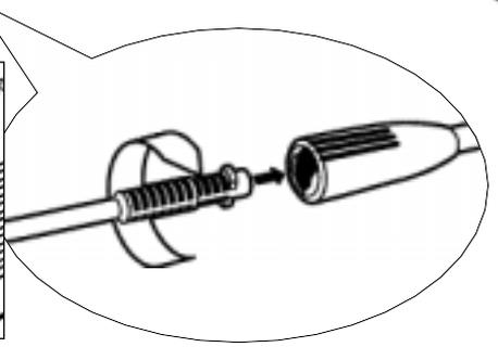
**Step 2** Insert the spray wand of your choice into the spray wand extension. Push in and turn clockwise to lock spray wand in place.
