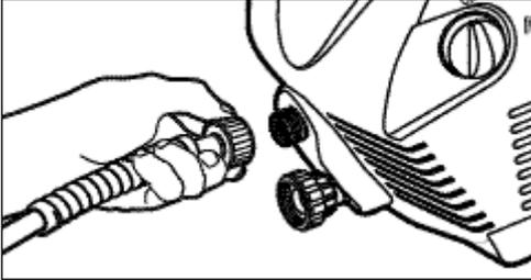
**Step 1** Connect the high pressure hose to the unit's high pressure outlet.
