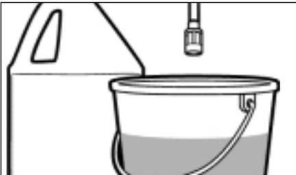
**Step 2** Fill a container with Karcher detergent. Place the filter end of detergent suction tube into the container.
