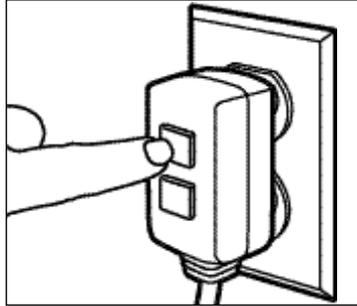
**Step 2** Press "TEST", then press "RESET" to assure proper connection to power.
