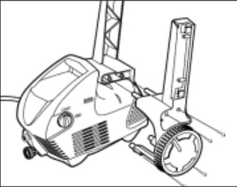
**Step 1** Slide each of the mobile adapter brackets to the pressure washer. Align the pegs and holes on the brackets. Insert the 4 screws and tighten as shown.
