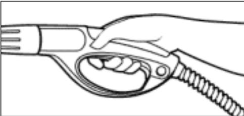
**Step 5** Plug the power cord into the power outlet. Trigger the gun to eliminate trapped air, wait for a steady flow of water to emerge from the spray nozzle.
