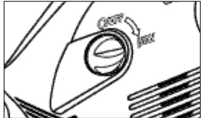
**Step 6** Turn on the pressure washer (I). The motor starts only if the trigger of the gun is pulled and shuts off when the trigger is released.
