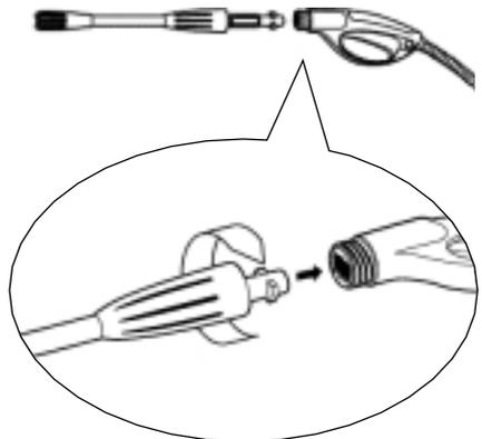
**Step 4** Slide the spray wand extension into the gun. Turn the wand collar clockwise onto the gun threads until tight.
