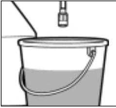
**Step 1** Remove detergent suction tube from container and insert into 1 gallon of fresh water. Siphon water at low pressure for one minute.
