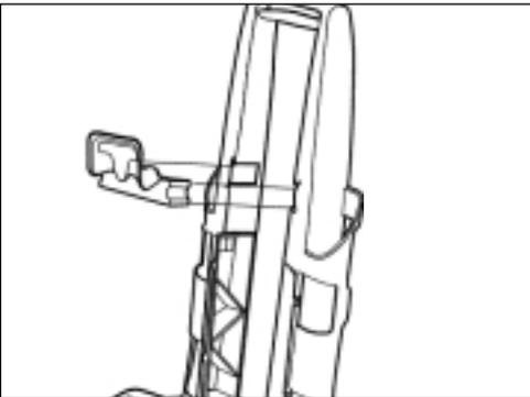
**Step 3** Slide the hose caddy into the handle slots and snap into place.
