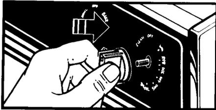
4. To replace, turn knob so off is at the top. Push control knobs straight back on.
