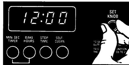
2. Turn the Set Knob to set the right time of day. Turning the knob clockwise increases the numbers, while turning the knob counter-clockwise decreases the numbers. The display will show the time you set in hours and minutes.
