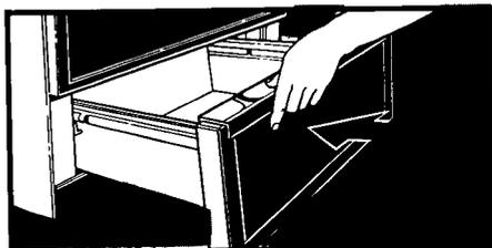
2. Lift drawer front. Then push in until the stops on the drawer slide rails have cleared the stops on the drawer guides. Lift drawer front again to clear the second stop. Slide drawer closed.
