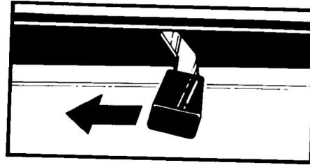
5. After the cleaning cycle is completed, the Auto Oven symbol and Self-Clean signal lights on the clock will go off. The display will show the time of day. **The oven door will stay locked and the Lock light will stay on until the oven cools down.** When the Lock light goes off, move the Lock Lever back to the left. **Do not force it.** Wait until it will move easily. This will turn off the Clean light. Turn the Selector and Temperature controls to OFF.
