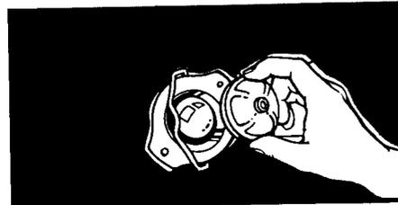
1. Remove the bulb cover in the back of the oven by pulling out and pushing the wire holder to the side.
