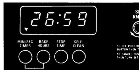
3. After setting the time you want, the signal light will stay on and the display will start counting down in seconds.
