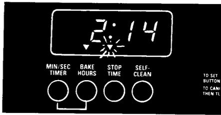
8. The Bake Hours signal light will stay on and the Stop Time signal light will flash. If you want to see the Stop Time, push the Stop Time button to see the baking time again.
