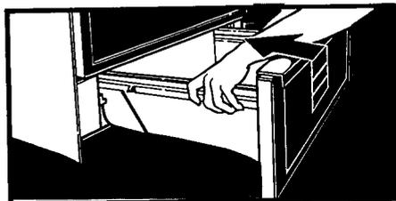
1. Fit ends of drawer slide rails into the drawer guides on both sides of opening.
