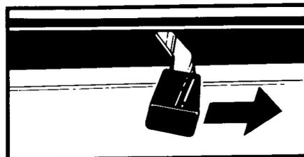
2. Move the Lock Lever all the way to the right. The Clean light will come on only when the lever is all the way to the right.
