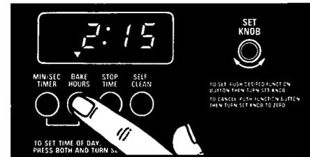
7. Set the clock for the desired amount of baking time: Push in the Bake Hours button and turn the Set Knob until the correct amount of baking time shows in the display. This example shows 2 hours, 15 minutes. Bake Hours can be set up to 11 hours, 59 minutes.
