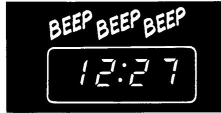
4. When the time is up, you will hear a beeping sound. Push the Min/Sec Timer Button to stop the beeping or the beeping will automatically stop after 1-2 minutes.
