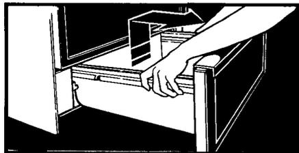
2. Lift back slightly and slide drawer all the way out.
