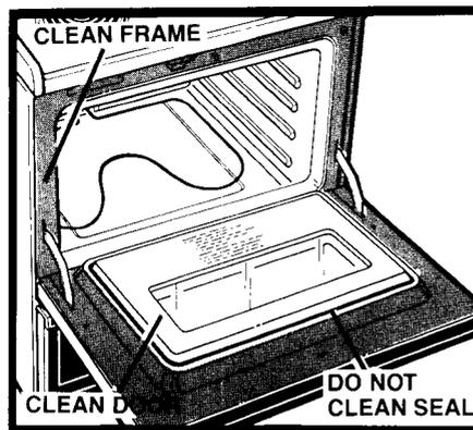
1. Clean the shaded areas by hand. They do not get hot enough during the Self-Clean cycle for soil to burn away. Use hot water and detergent or soapy steel wool pad on...
