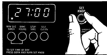
2. Turn the Set Knob until the desired time shows in the display. Turning the knob clockwise increases the numbers, while turning the knob counterclockwise decreases the numbers.
