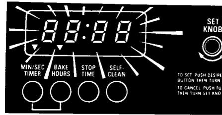
After the sequence is completed, 4 eights and the Min/Sec Timer and Bake Hours signal lights will flash. The flashing means that the clock is ready to be set.
