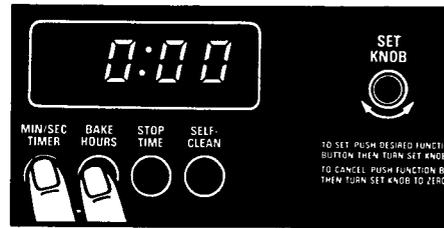
1. Push in both the Min/Sec Timer and the Bake Hours Buttons. "0:00" will show in the display and the signal lights will go off.
