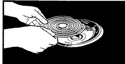
2. Pull the surface element straight away from the receptacle.
