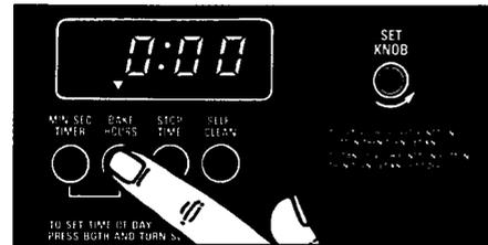
8. **To stop oven before the programmed time,** push in the Bake Hours button and turn the Set Knob counterclockwise until the display shows "0:00." The display will return to the time of day. Turn the Selector and Temperature controls to OFF.
