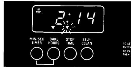
6. The Bake Hours signal light will stay on. The Stop Time signal light will flash and the Auto Oven symbol light will come on. **The display will count down in minutes.** If you want to see Stop Time, push the Stop Time button. Push Bake Hours button to see the baking time again.
