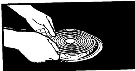
3. Push the surface element terminal into the receptacle. When the terminal is pushed into the receptacle as far as it will go, the surface element will fit into the trim ring.
