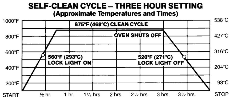
Notice that heating stops when the 3-hour setting is up, but that it takes longer for the oven to cool down enough to unlock.
