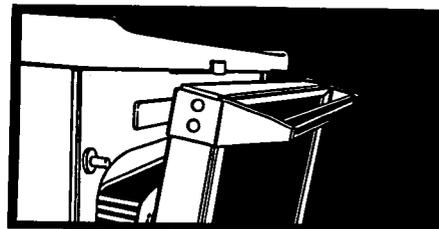
3. Close the door to the Broil Stop position, (open about 4 in., 10.2 cm). The door will stay open by itself.
