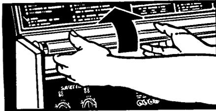
2. Grasp the fluorescent tube at both ends. Turn the tube away from you until both ends come out of the receptacles.
