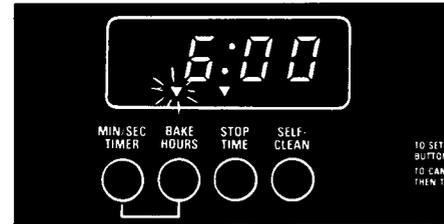
6. The display will show the time you set. The Stop Time signal light will stay on. The Bake Hours signal light will flash.
