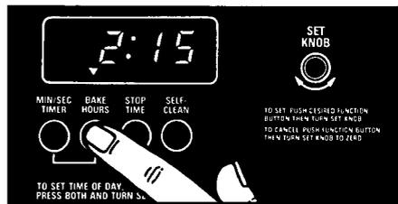
5. **Set the clock for the desired amount of baking time.** Push in the Bake Hours button. Then turn the Set Knob until the correct baking time shows in the display. This example shows 2 hours, 15 minutes. Bake Hours can be set for up to 11 hours, 59 minutes.
