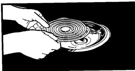
2. Hold the surface element as level as possible with the terminal just started into the receptacle.
