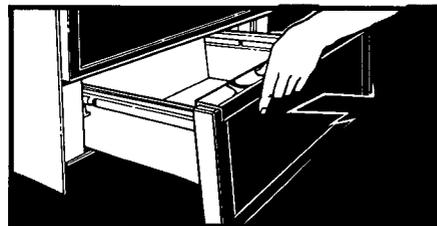
1. Pull drawer straight out to the first stop. Lift front and pull out to the second stop.
