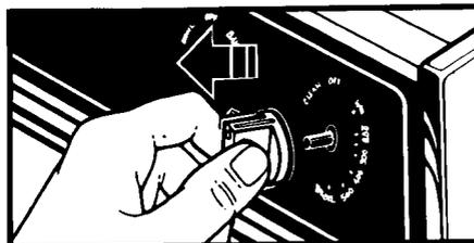
1. First make sure the control knobs are set to OFF. To remove, pull knobs straight off.
