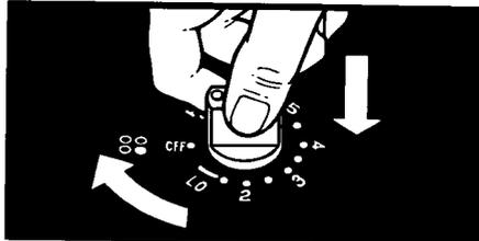
**WARNING: To avoid burns and possible electric shocks, make sure all controls are OFF and the elements are COOL before cleaning.**
