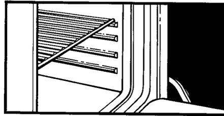
1. Position the rack before turning the oven on. See broil chart in the "Cooking Guide" or a reliable cookbook for recommended rack positions.
