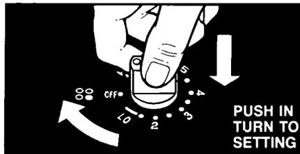
**Control knobs must be pushed in before turning them to a setting.** They can be set anywhere between HI and OFF.
