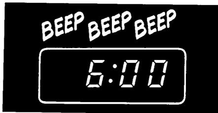
10. When baking is complete, the oven will shut off automatically. You will hear a beeping sound. Push the Bake Hours button to stop the beeping, or the beeping will stop automatically in 1-2 minutes.
