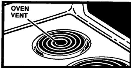
The oven vent is located under the right rear surface element. When the oven is on, hot air and moisture escape from the oven through this vent. Poor baking can result if this vent is blocked. When using the oven, **do not** use oversized pans or other items that might block the oven vent.
