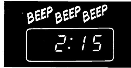
7. **At the end of the selected baking time,** the oven will shut off automatically. You will hear a beeping sound. Push the Bake Hours button to stop the beeping or the beeping will stop automatically after 1-2 minutes. Turn the Selector and Temperature controls to OFF.
