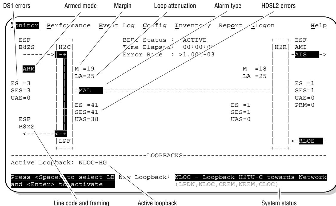
Figure 11. Monitor Screen - Active Loopback with Alarms
