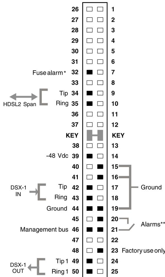
\* Fuse alarm is normally floating and at -48 Vdc when activated.
