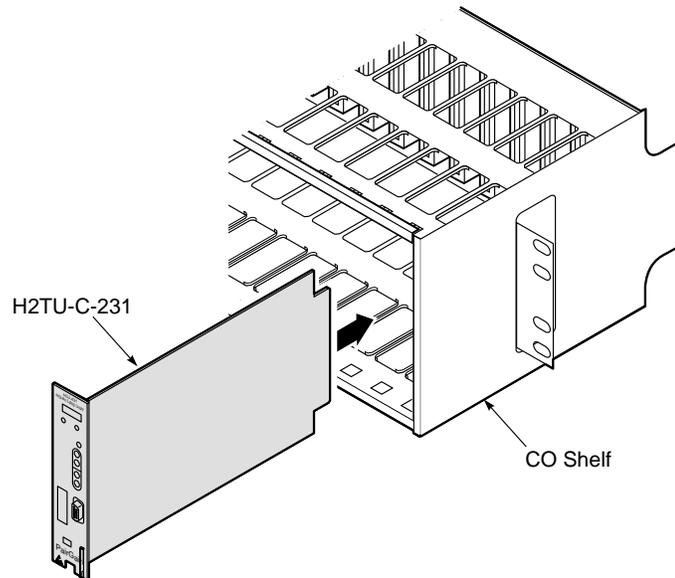
*Figure 2. Installing the H2TU-C-231 List 2 into a Shelf*
