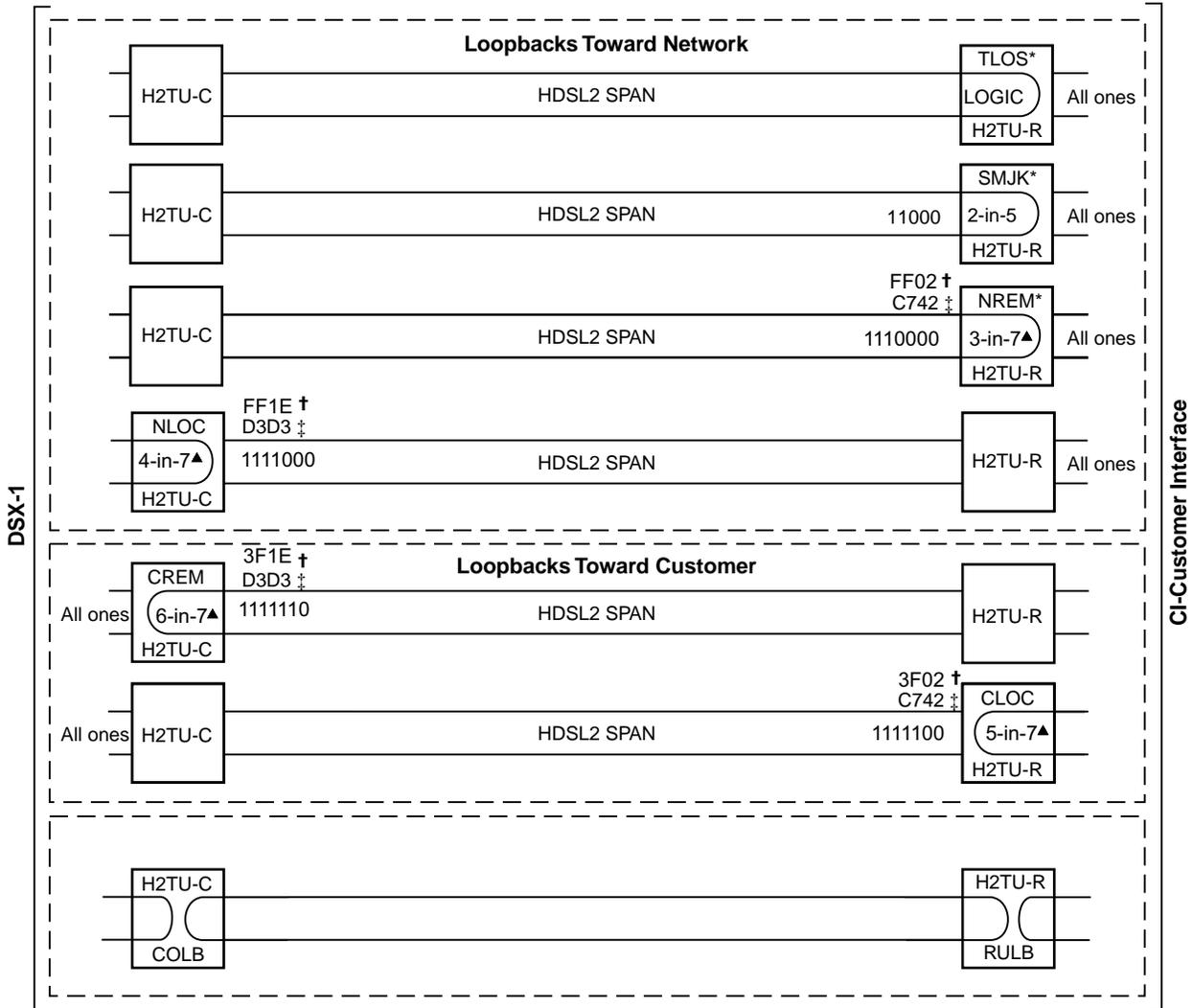
\* Set the NLBP option to AIS to send AIS (indicated by an all ones pattern) for any network loopback.
