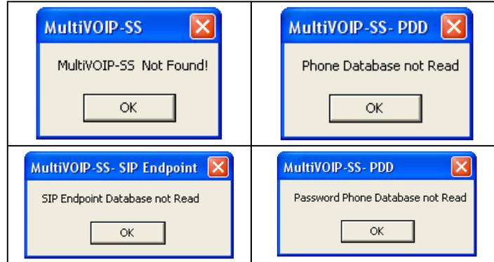
In this case, the MultiVOIP is simply disconnected from the network. For instructions on MultiVOIP cable connections, see the Cabling section of Chapter 3.
