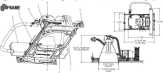
Complete Fixture consists of Frame-In Kit and Reflector Trim. Select each separately.
