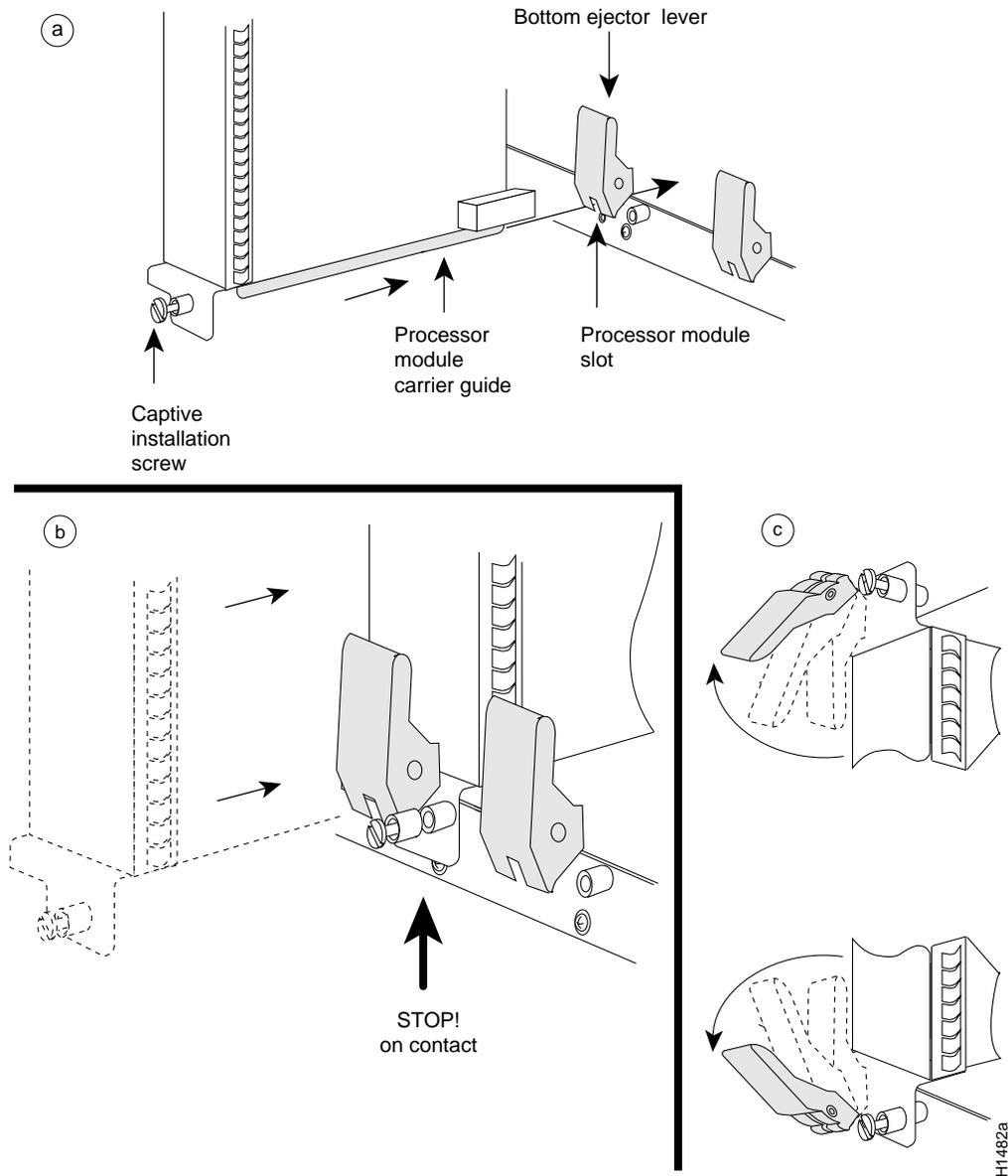
**Step 3** Place the back of the RSP7000 in the 7000 RSP slot and align the notches along the edge of the carrier with the grooves in the slot. (See Figure 4a.)
