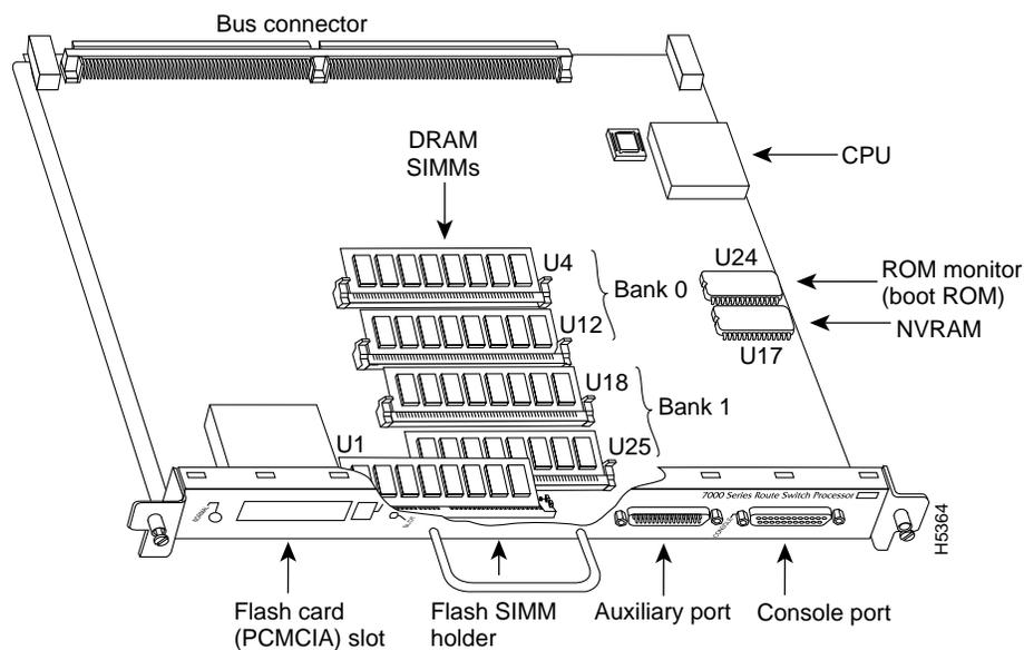
The SIMM sockets use the thumb tabs that are often used in PCs and other computer equipment. Each RSP7000 SIMM socket has two metal retaining springs, one at each end. (See Figure 7 on page 31.) When a SIMM is fully seated in the socket, the retaining springs snap over the ends of the SIMM to lock it in the socket.
