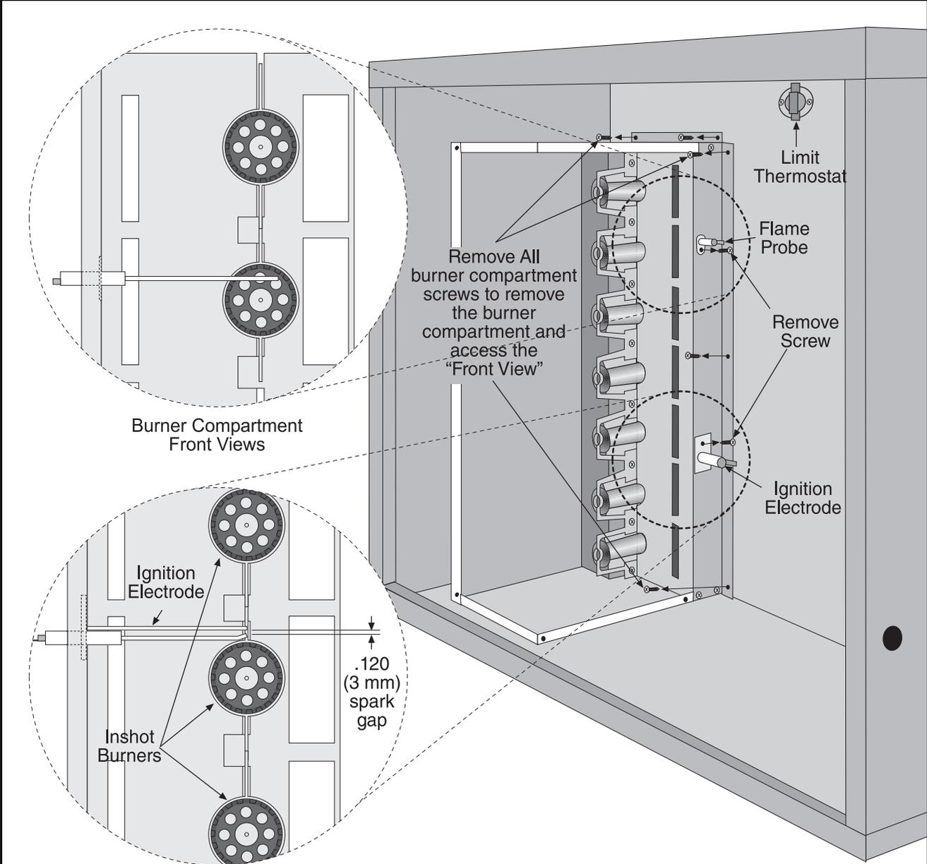
To replace the electrode or flame probe, remove the electrical lead and screw. Pull out from mounting. Refit in reverse ensuring that the gap to burner is as shown in the front view of the burner compartment.
