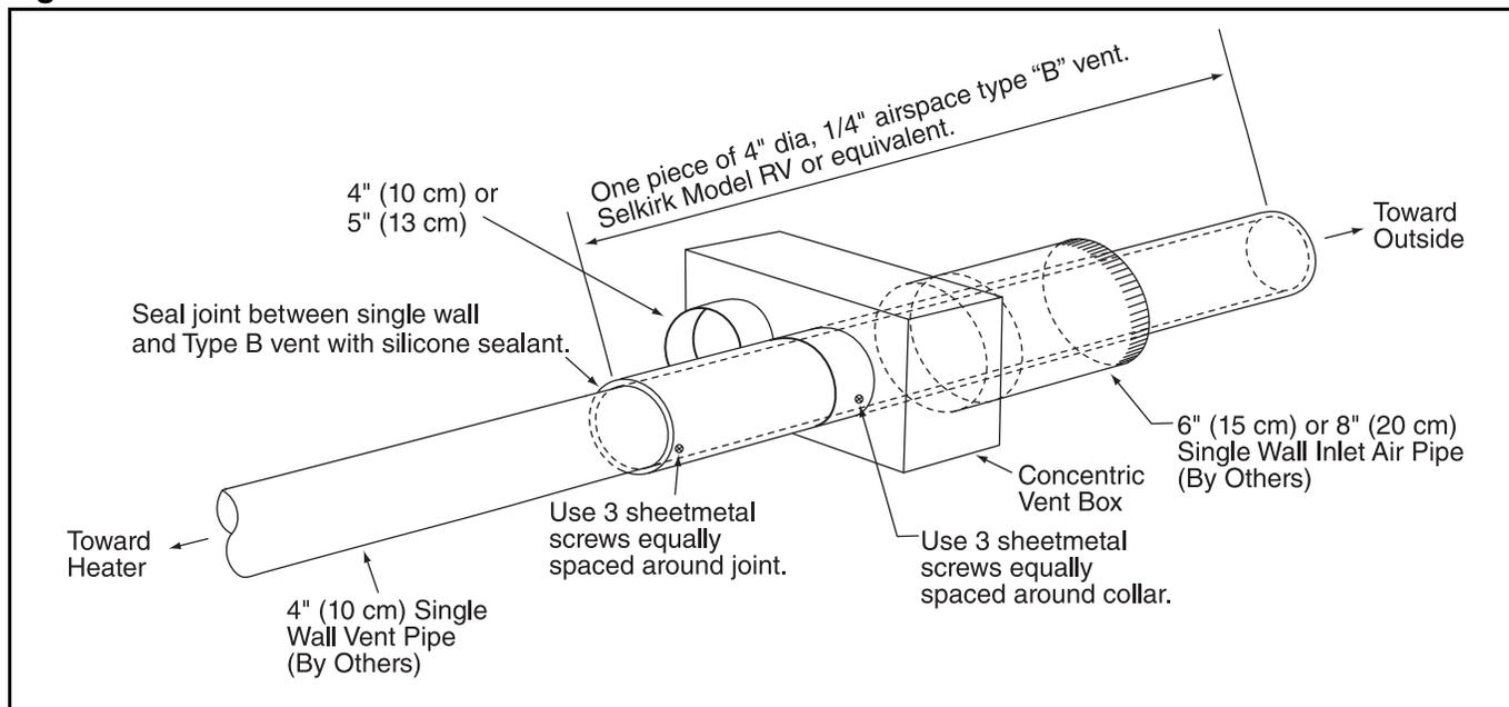
**Figure 8: Concentric Vertical and Horizontal Vent Termination - Separated Combustion Heater**
