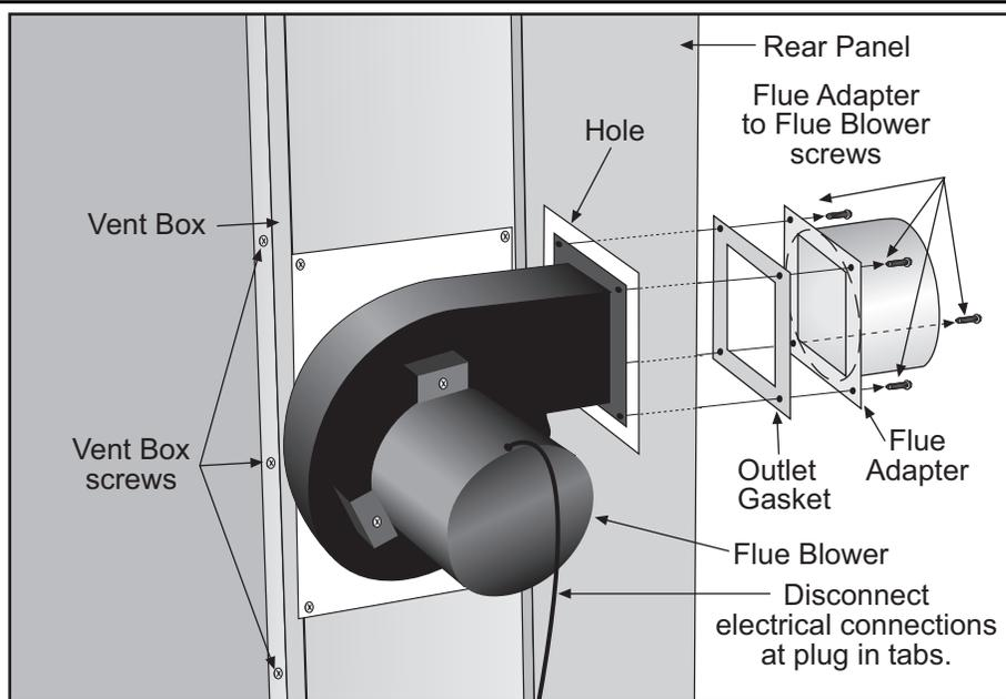
Remove screws securing outlet flange to the flue adapter.
