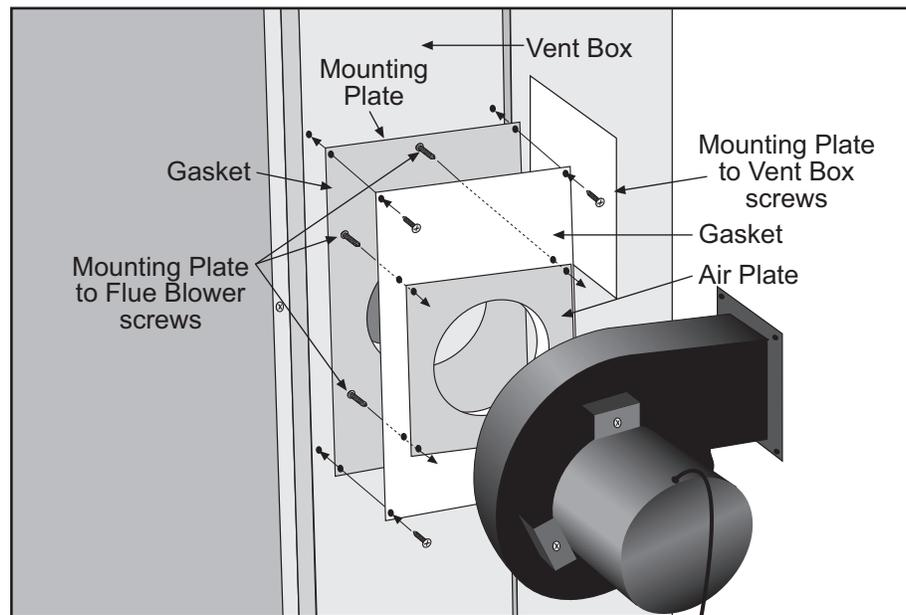
Remove screws securing flue blower mounting plate to vent box.
