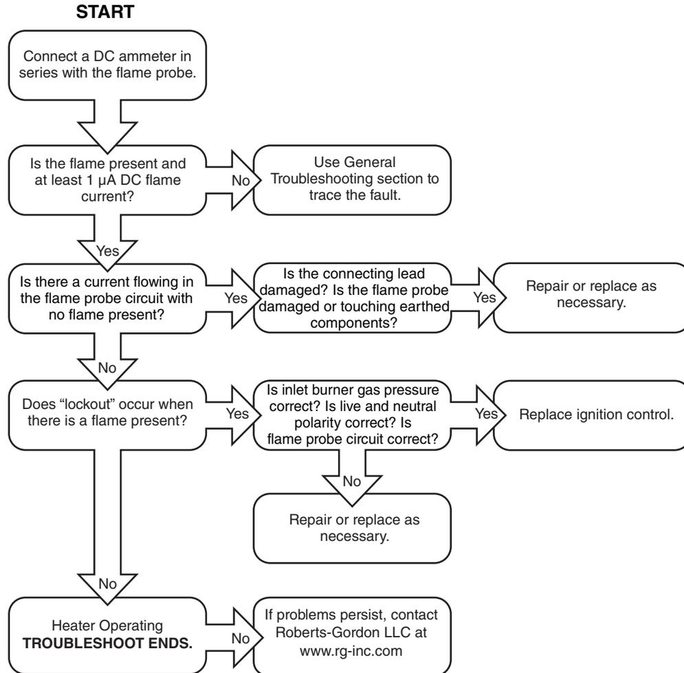
**NOTE:** Minimum flame probe current 1  $\mu\text{A}$  DC. Typical flame probe current 3-5  $\mu\text{A}$  DC.
