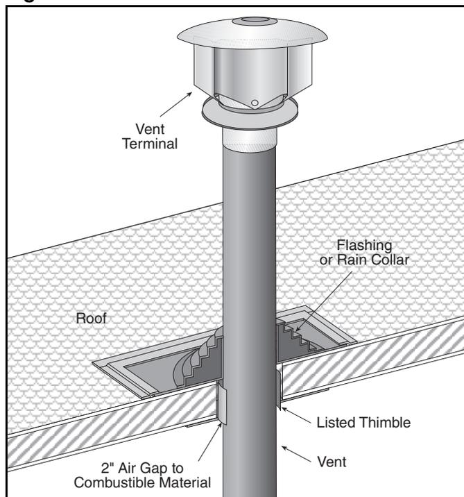
**Figure 4: Standard Vented Heater - Vertical and Horizontal Vent Termination**
