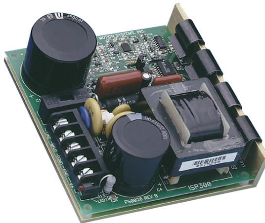
Figure 2.2.1: IMS ISP300 Switch Mode Power Supply
