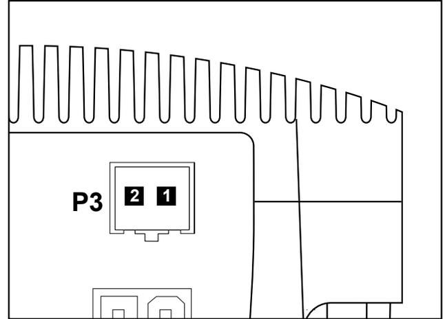
Figure 1.2.3: P3 — 2-Pin Locking Wire Crimp Pin Configuration
