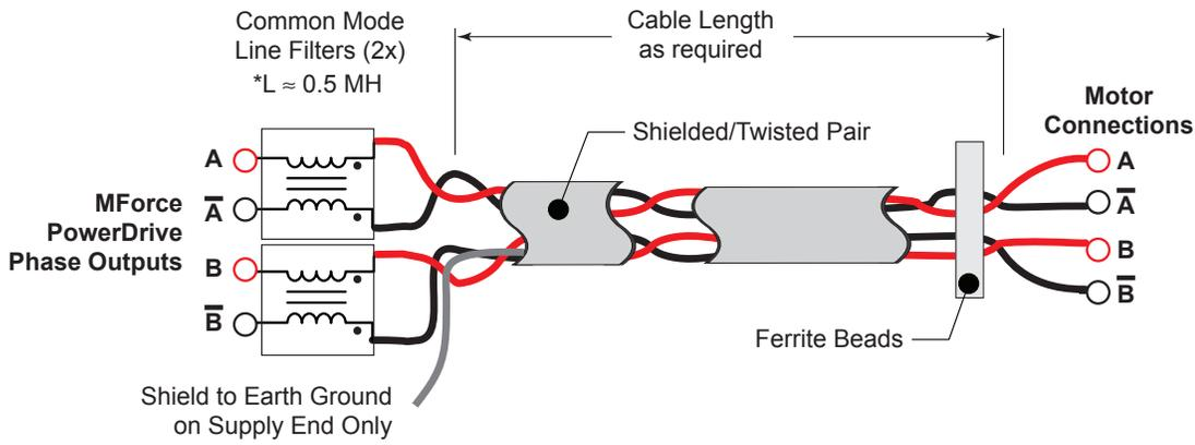
\* 0.5 MH is a typical starting point for the Common Mode Line Filters. By increasing or decreasing the value of L you can set the drain current to a minimum to meet your application's requirements.
