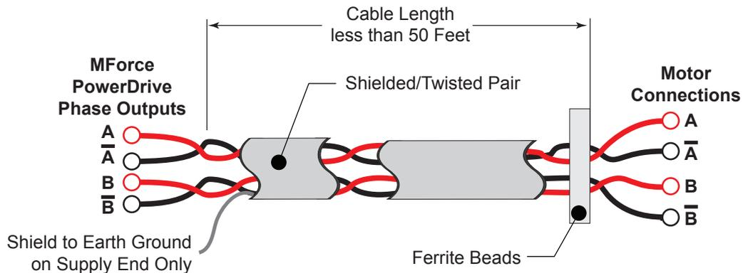
Figure 2.3.7: Motor Cabling Less than 50 Feet
