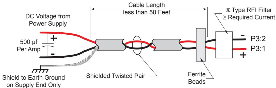
Figure 2.2.3: DC Cabling - Under 50 Feet
