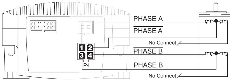
Figure 2.3.4: 6 Lead Half Coil (Higher Speed) Motor Connections
