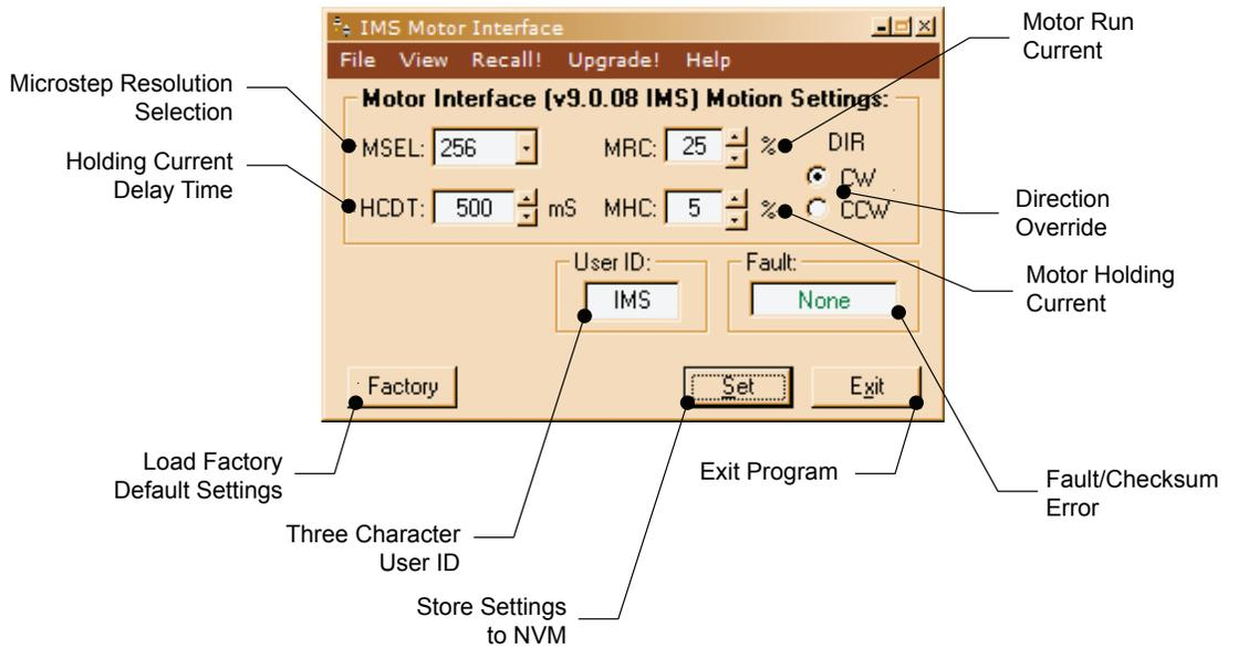
Figure 2.6.7: SPI Motor Interface Motion Settings Screen
