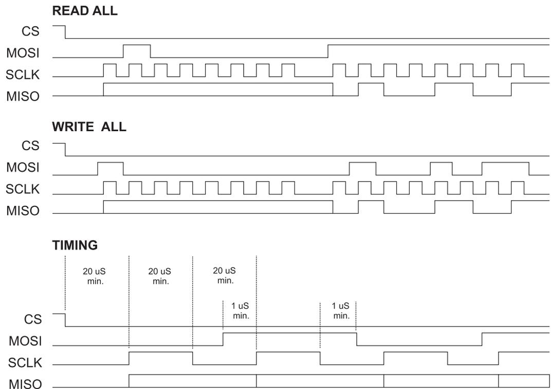
Figure 2.7.1: SPI Timing
