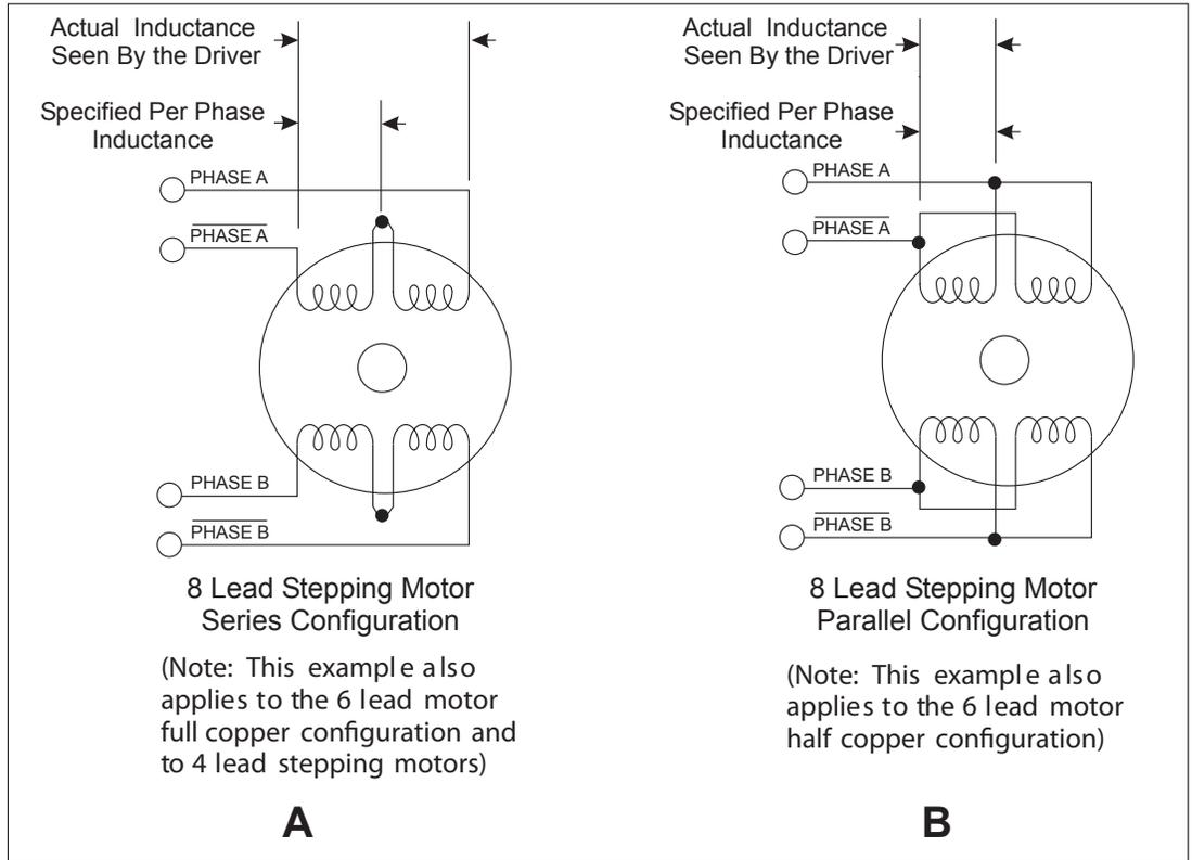
Figure 2.3.1 A & B: Per Phase Winding Inductance
