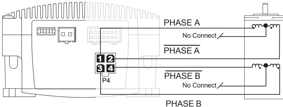
Figure 2.3.5: 6 Lead Full Coil (Higher Torque) Motor Connections
