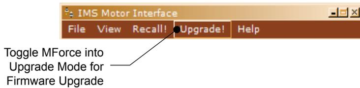
Figure 2.6.5: SPI Motor Interface Upgrade Menu
