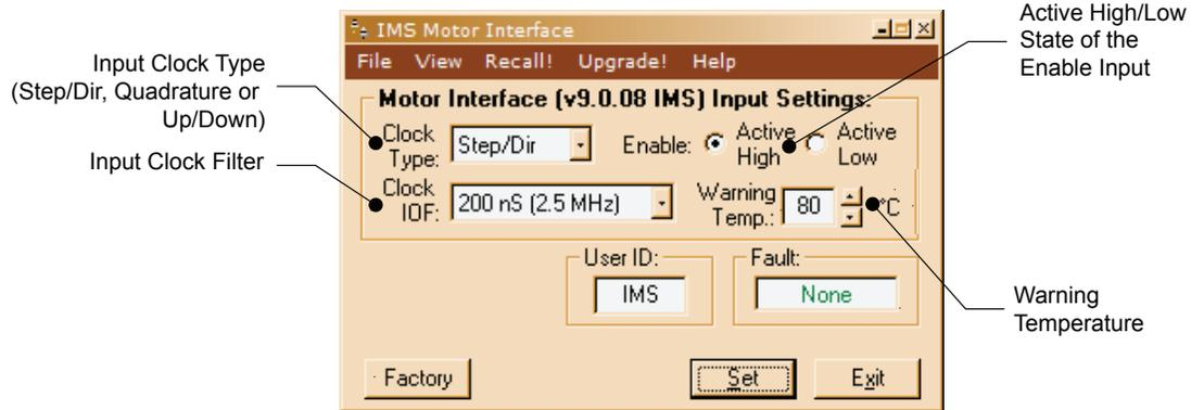
Figure 2.6.8: SPI Motor Interface I/O Settings Screen
