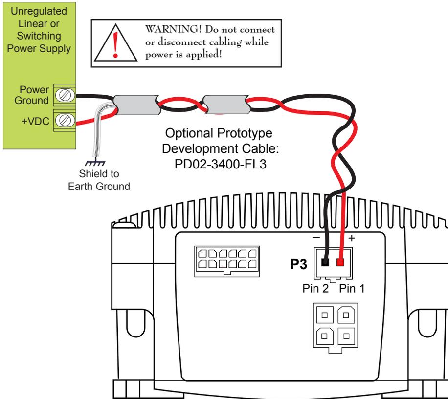
**WARNING! DO NOT** connect or disconnect power leads when power is applied! Disconnect the AC power side to power down the DC power supply.
