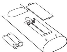
Remove the back cover to insert the batteries, make sure they are inserted the right way round.
