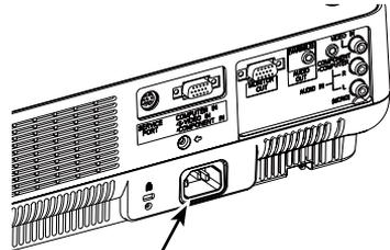
Connect the AC power cord (supplied) to the projector. The AC outlet must be near this equipment and must be easily accessible.
