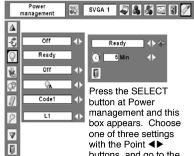
Press the SELECT button at Power management and this box appears. Choose one of three settings with the Point ◀▶ buttons, and go to the timer with the Point ▲▼ buttons and set time with the Point ◀▶ buttons.
